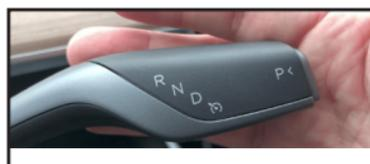
With foot on the brake, move the lever to drive, and/or up for reverse. To park the vehicle, press the button inward on the right shifter.
